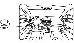
$(1) \ \mbox{The buzzer is suggested to install under the left side of the steering wheel;}$
