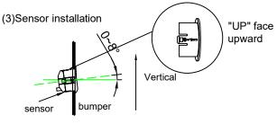
a.By using different sensor masker to fit the bumper, make sure the angle between 0~8°;
